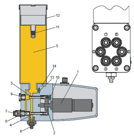
The rotational movement of an electric motor 1 is converted via a swash plate 2 into a lifting movement of the delivery pistons 3 and 4. In the suction position (piston 4) the medium is drawn in from the cartridge 5, in the pressure position (piston 3) the medium is pumped towards the outlet.
