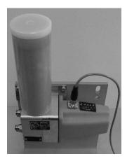
6. When using oil as a lubrication medium, the unit can also be turned over after the filling process (only for use with follower piston), so that the tank points downwards and the outlets point slightly upwards at an angle. Then actuate the unit until the medium emerges bubble-free.
