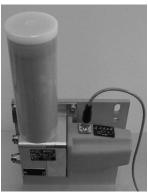
3. Then position the cartridge and screw it on tightly. Ensure that the O-ring is correctly seated.
