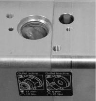
3. For the next steps, the lid should be removed from the cartridge. Then screw the empty cartridge into the pump body. The O-ring 18,0x3,5 for cartridge sealing must be located in the thread run-out of the res-ervoir. The cartridge must be tightened firmly to ensure a sealing effect between the cartridge and the pump. During the screwing-in process, the air trapped in the cartridge pushes the follower piston slightly upwards.
